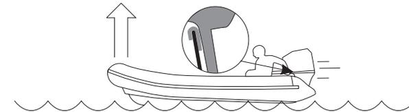
An outboard tilted too close to the transom will drive the bow section too deep into the water which ends up in loss of speed and/or cavitation.
