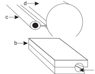
The seat rails (c) are connected to the inner sides of inflatable tubes (d) of your boat. The seat holders (b) are connected to the lower side of the seats. Insert the seat rails c into the holes a of your seat holders on the both sides of the boats equally and move the seat to the proper position.
