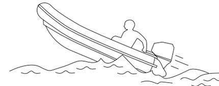
There is another less common known hazardous result from allowing your boat to launch off a wave or wake. If the bow of your boat pitches down far enough while airborne, upon water contact it may penetrate under the water surface and submarine for an instant. This will bring the boat to a nearly instantaneous stop and can send the occupants flying forward. The boat may also steer sharply to one side.
