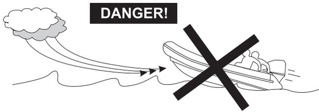
Wind and wave conditions can be highly dangerous for your inflatable. You can easily be flipped over if the load in the boat is not distributed in the bow of the boat and wind and tide are against. Especially the models with inflatable floor should be driven carefully in headwind and waves.
