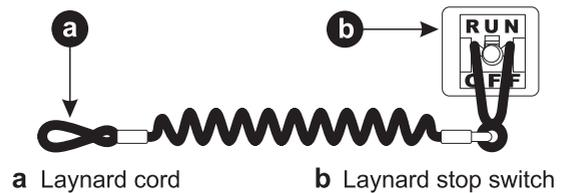
The purpose of a lanyard stop switch is to stop the engine when the operator moves far enough away from the operator's position to activate the switch. This would occur if the operator accidentally falls overboard or moves within the boat a sufficient distance from the operator's position. While activation of the lanyard stop switch will stop the engine immediately, a boat will continue to coast for some distance depending upon the velocity and degree of any turn at shut down.
