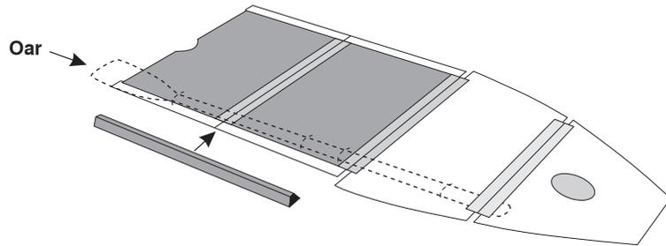
To make the installation of the stringers easier **we recommended putting an oar under the bottom** of the boat. This lifts up the floorboards to have easier access to put the stringers on the sides of the floor.
