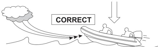
Distribution of load and weight take the bow down to a safe situation. The anti-cavitations plate on the engine should be about 30-50 mm under the bottom of the transom.
